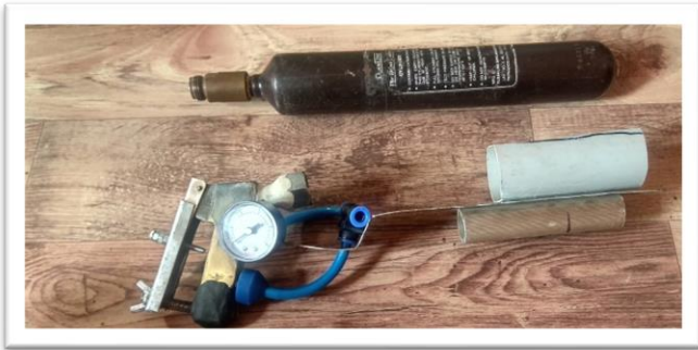
Fig.8: Pressure Regulator & Pressure Gauge
